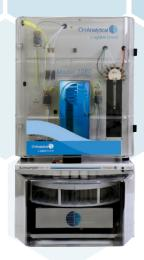
Figure 1. OI Analytical 1080 TOC Analyzer
